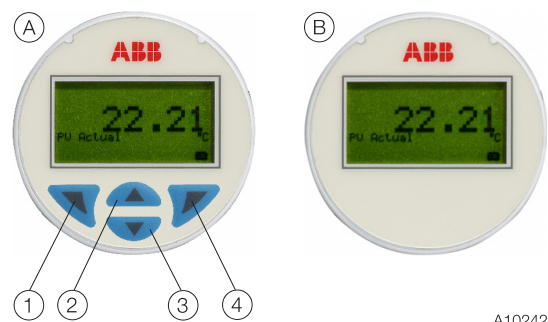
Fig. 10: (A) LCD indicator type A (B) LCD indicator type AS ① Exit / Cancel ② Scroll back ③ Scroll forwards ④ Select
