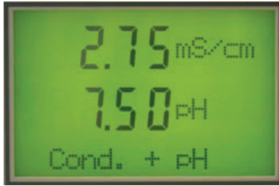
Simultaneous conductivity and pH measurement
